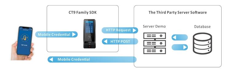
Developer is able to customize and display specific background image with TEXT information on 3.5" touch screen controlled by server via HTTP command for user to view the real time information, announcement.
