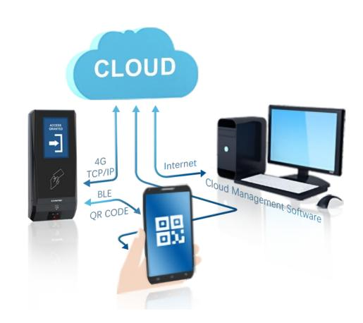
As online reader, CT9 PRO/CT9E use standard HTTP/HTTPs to get bio-direction communication between CT9 PRO/CT9E and third party cloud server. It works as CLIENT to automatically detect if server is online. When CT9 PRO/CT9E establishes a connection with the cloud server, it can automatically receive HTTP commands from the cloud server or actively send HTTP commands to the cloud server. Each device contains a MAC address to avoid IP conflict for smart devices remote management.
