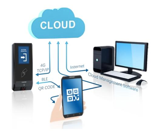
As online reader, CT9 PRO/CT9E use standard HTTP/HTTPs to get bio-direction communication between CT9 PRO/CT9E and third party cloud server. It works as CLIENT to automatically detect if server is online. When CT9 PRO/CT9E establishes a connection with the cloud server, it can automatically receive HTTP commands from the cloud server or actively send HTTP commands to the cloud server. Each device contains a MAC address to avoid IP conflict for smart devices remote management.
